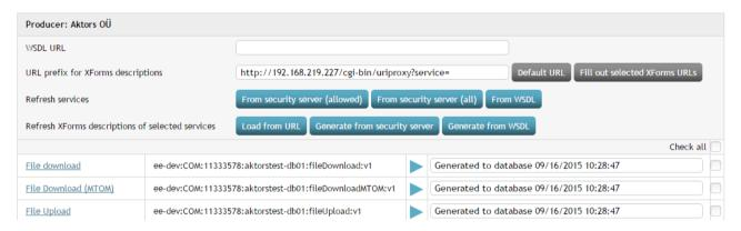
The system also downloads WSDL descriptions for each service to extract human-readable service names from them. Those names are displayed in the first column of service list. The x-road identifier consisting of X-road instance, member class, member code, subsystem code, service name and service version (all separated with a colon), are displayed in the second column.
